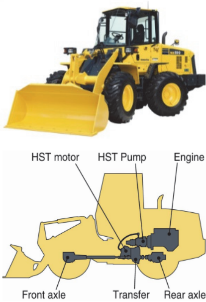
Fig. 1 Schematic of a wheel loader [1]
