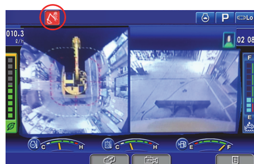
Fig. 12 Lock lever lock status indication
