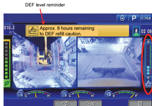
Fig. 17 DEF level indication
