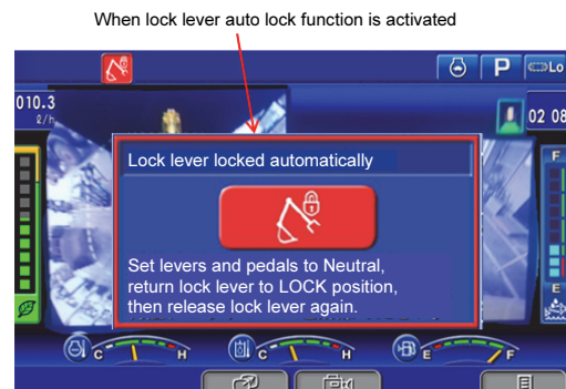
Fig. 11 Display on the monitor when the lock lever auto lock function is activated
