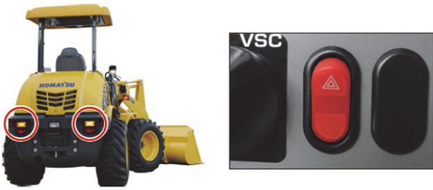
Fig. 6 Hazard Lamp (cited from in-house document)
