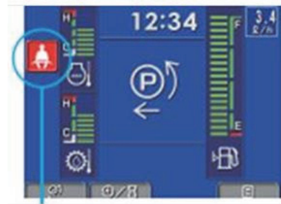
Fig. 4 Alarm for Not-fastening Seat Belt (cited from in-house document)
