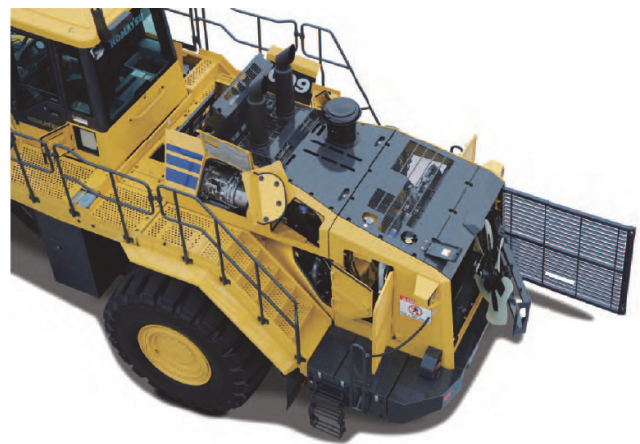
Fig. 12 Swing-type Fan and Engine Exterior Door
