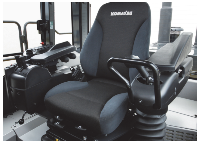
Fig. 7 Operator Seat Integrating Work Machine into Advanced Joystick Steering System
