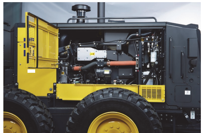
Fig. 7 Arrangement under the engine hood
