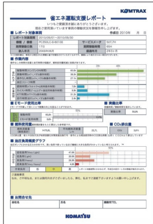
Fig. 21 Report of support for energy-saving operation
