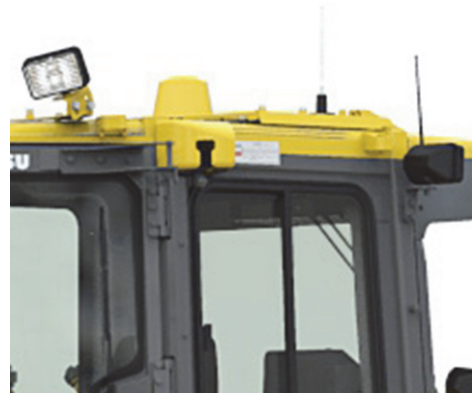
Fig. 17 Roof top antenna
