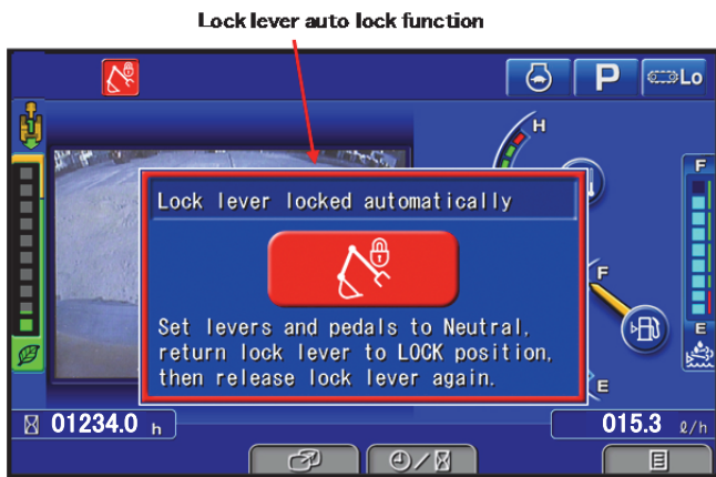
Fig. 8 “Lock lever auto lock active” message on the monitor screen (Source: Komatsu data archive)
