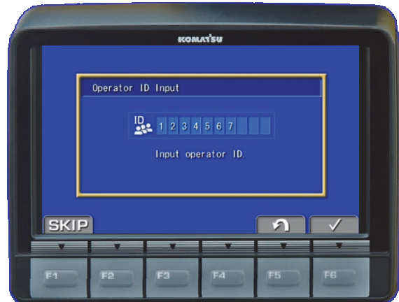
Fig. 10 Operator authentication screen (Source: Komatsu data archive)
