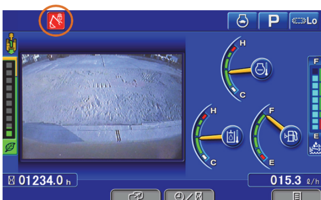
Fig. 9 Lock lever locked status indication (Source: Komatsu data archive)
