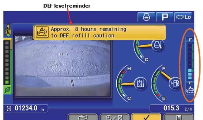
Fig. 11 DEF level indication (Source: Komatsu data archive)
