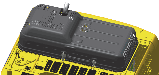
Fig. 12 Press molded one-piece engine hood
