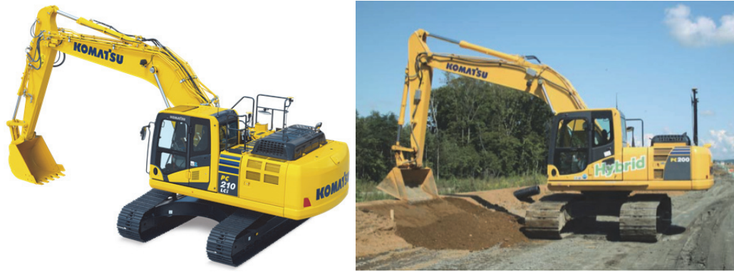
Fig. 1 PC210LCi-10/PC200i-10 External view (left) Conventional MG hydraulic excavator (right)
