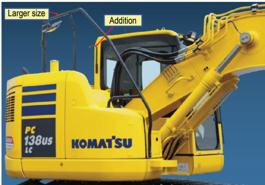
Fig. 13 Handrail for preventing a fall from the machine cab
