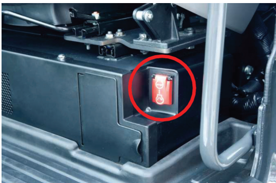
Fig. 14 Secondary engine stop switch
