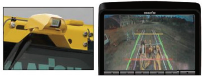
Fig. 11 Rear checking camera and camera image
