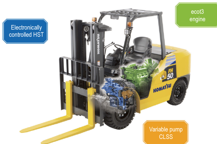
Fig. 2 General view of FH50-1
