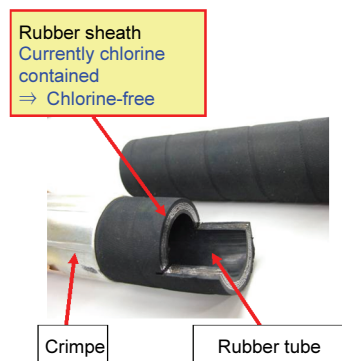
Fig. 3.1 Rubber Sheath Needs to be Chlorine-free
