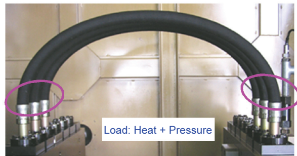
Fig. 4.2 Durability Evaluation under Heat and Pressure
