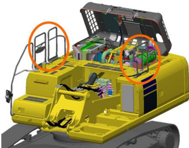
Fig. 14 Handrails to prevent falling from the machine cab (Source: In-house material)
