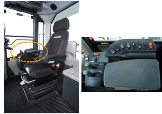
Fig. 11 Electric work equipment levers and right console mounted near the operator’s seat
