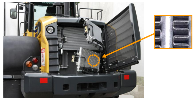
Fig. 18 Rear grille and cooling unit of the swing-out type
