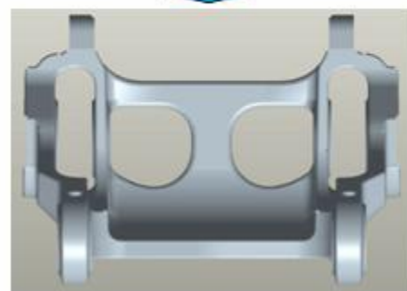
(d) Shape as a result of optimization
