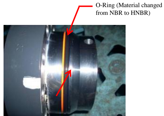
Fig. 8 Application example (Cylinder head contact surface)
