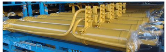
Photo 3 Appearance of the hydraulic cylinder
