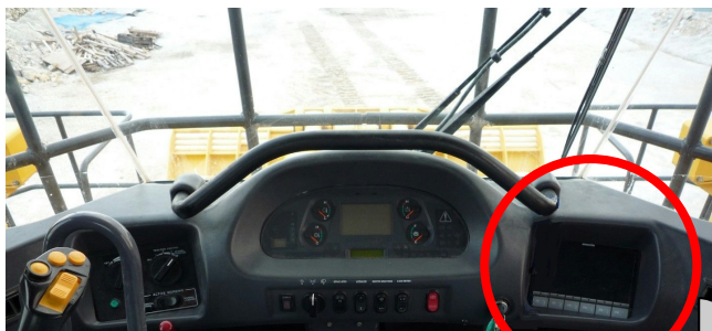
Fig. 17a Monitor panel
