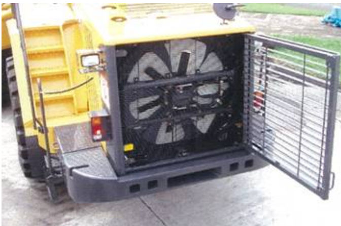
Photo 7 Hydraulic drive fan
