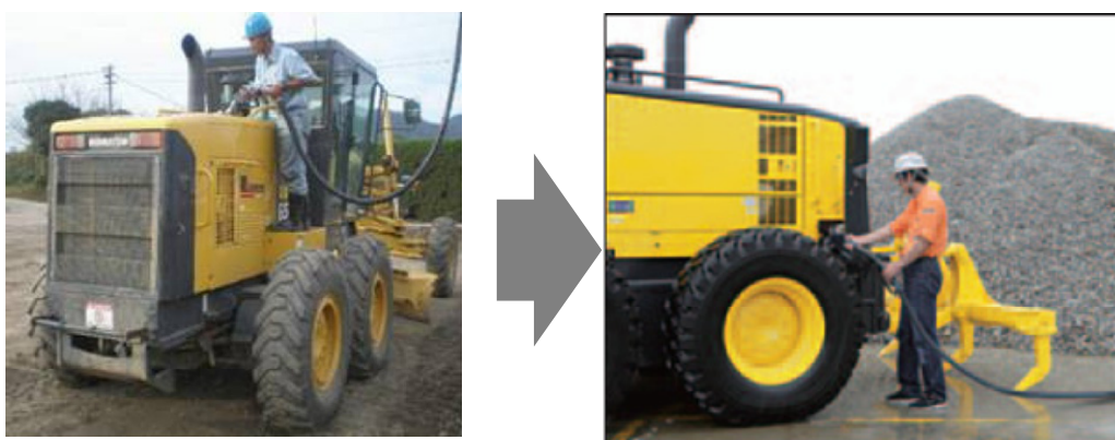
Fig. 3 Improvement in fuel supplying method
