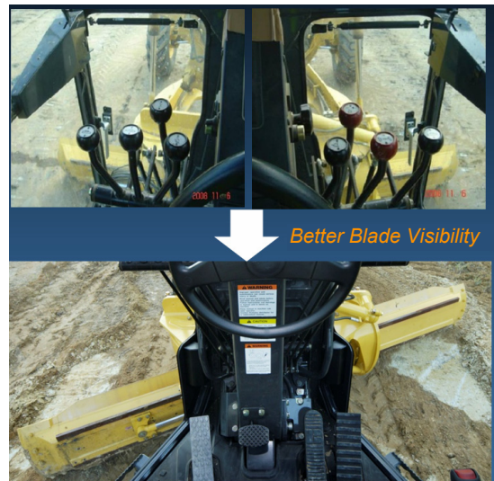
Fig. 5 Comparison of visibilities of work equipment between former and new models
