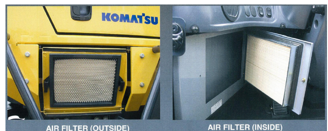
Fig. 9 Inside and outside air filters
