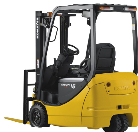
Photo 2 FB15M-12(E3) 1.5 counter three-wheel type
