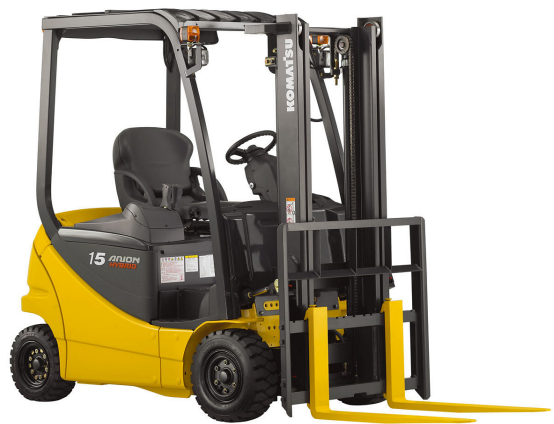
Photo 3 FB15HB-12 (HYBRID) 1.5-ton battery hybrid forklift
