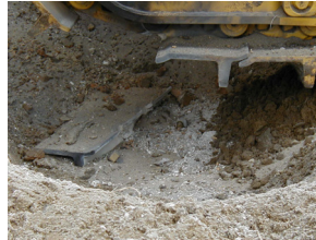
Photo 6 Fallen shoe, bent bolt
