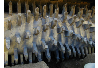
Photo 7 Chipped bit, fallen bit
