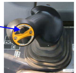
Photo 3 Load control switch
