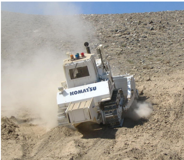
Photo 8 Demining on a steep inclined surface in Afghanistan
