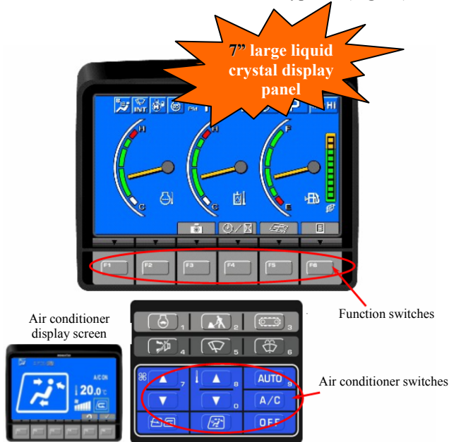
Fig. 11 Color multi-monitor screen and function switches
