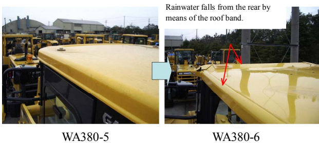
Fig. 17 Improved roof shape
