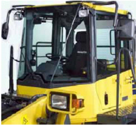
Closed pressure type large pillarless cab featuring wide visibility
