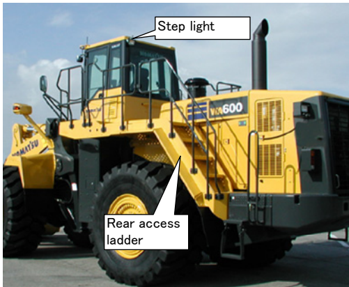
Photo 3 Rear access ladder
