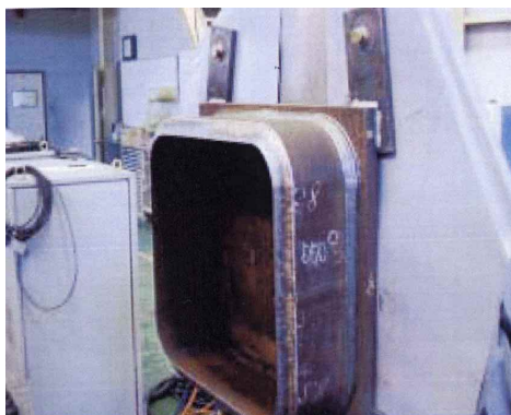
Fig. 7 Example cutting of column steel
