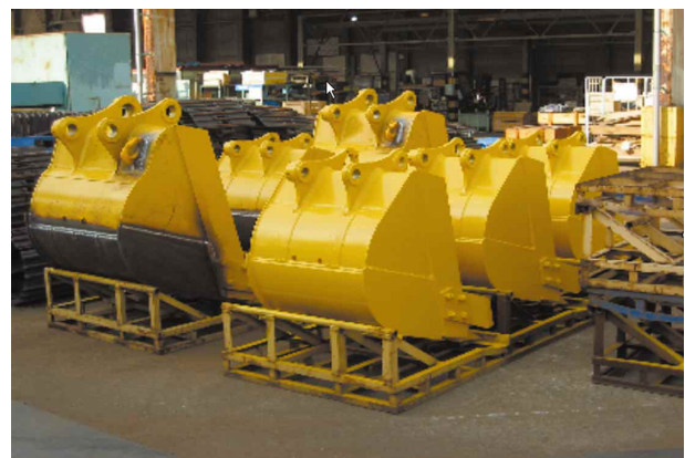
Photo 1 Example of repaired buckets
