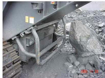
Photo 6 Conveyor tail section
