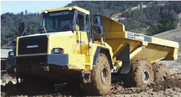
Fig. 3 Articulated dump truck
