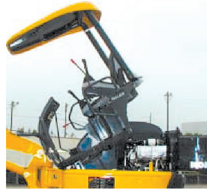
Photo 7 Machine with its floor tilted up
