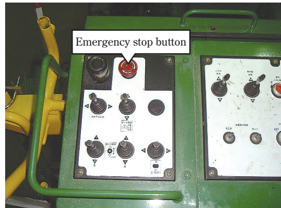
Photo 5 Emergency stop button
