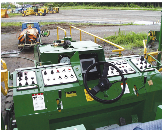
Photo 4 Operation panels at both sides of operator's seat
