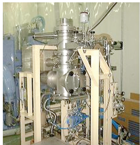
Photo 1 Equipment for plasma treatment of powder
