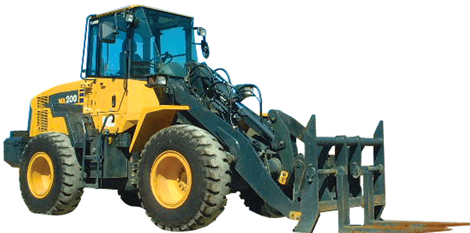
Photo 1 Newly-developed wheel loader with AC linkage
