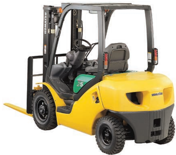
Photo 2 2-ton Forklift Trucks
