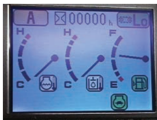
(c) LCD subjected to reflection-reducing treatment There is no problem in visibility of display, although the portion in which the fluorescent lamp is reflected is somewhat whitened.
