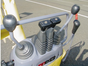
Similarly to upper models, right and left independent travel levers are installed so that operator can clearly distinguish operations of both tracks.
