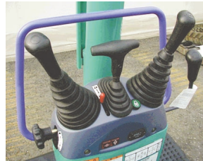
Operator moves single lever forward and back and twist it to control travel.
