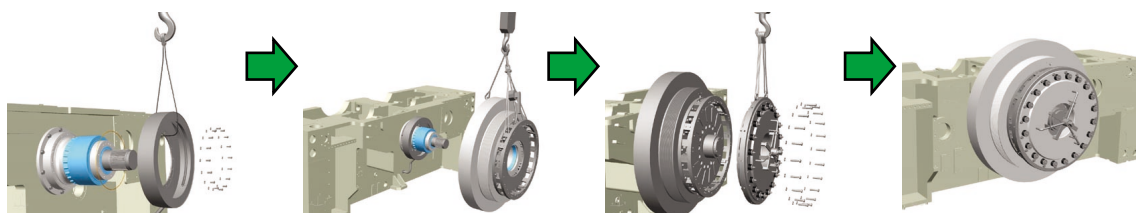
Fig. 2 An instance of digital assembly showing clutch installation
