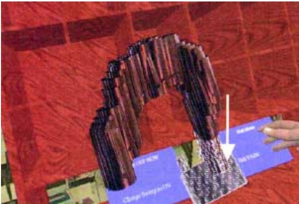
Fig. 6 Loci of movement and check of interference
