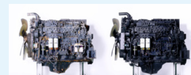
Left: Engine before Reman Right: Engine after Reman
