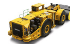
LHDs (load, haul, dump machines)
