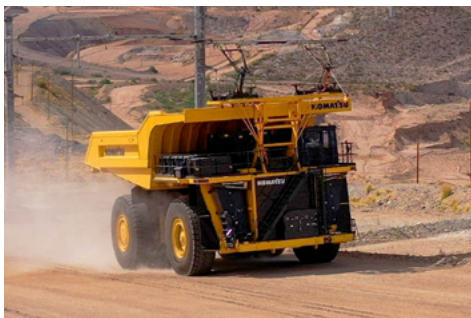
Battery-electric trolley mining truck (Concept machine)
