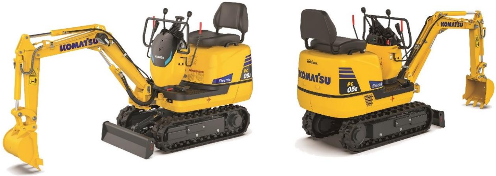
New electric micro excavator powered by a swappable mobile battery, “PC05E-1”
