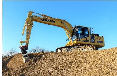
Hydraulic excavator (Crawler-type)
