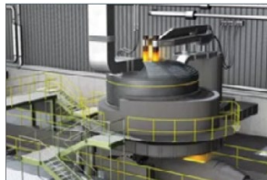
Rendering of next-generation melting furnace using superinsulation
