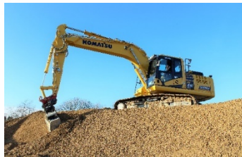
Hydraulic excavator (Crawler-type)
