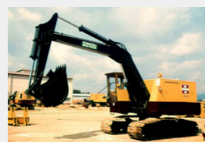
Hydraulic Power Excavator 15H-1
