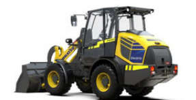
Fully electric wheel loader (concept machine)
