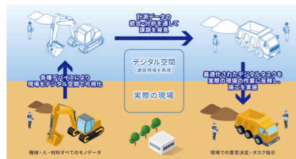
Concept diagram of DX Smart Construction solution with a digital twin
