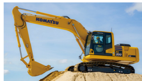
PC200-10M0 hydraulic excavator with urban civil engineering specifications (CE series)
