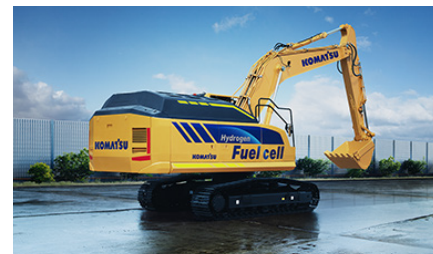
Middle-sized hydraulic excavator equipped with a hydrogen fuel cell (concept machine)
