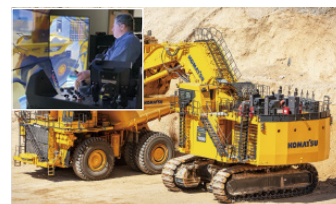
Collaborative operation by unmanned dump truck and ultra-class teleoperated hydraulic excavator (development completed in March 2023)
