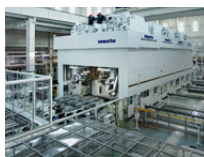
Large size AC servo presses for forming automotive body panels
