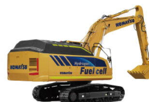
Medium-sized hydraulic excavator equipped with a hydrogen fuel cell (concept machine)
