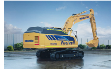
Medium-sized hydraulic excavator equipped with a hydrogen fuel cell (concept machine)
