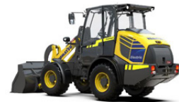
Fully electric wheel loader (concept machine)
