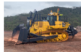
Large-scale ICT bulldozer for mining, D375Ai-8 teleoperation model
