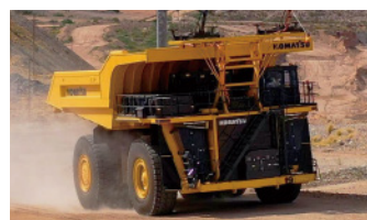
Battery-powered haul truck (concept machine)
