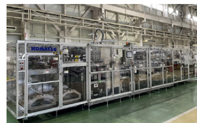
IL221-7 cell tab molder with slitter
