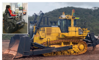
Large-scale ICT bulldozer for mining D375Ai-8 teleoperation model (commercial operation commenced in May 2023)
