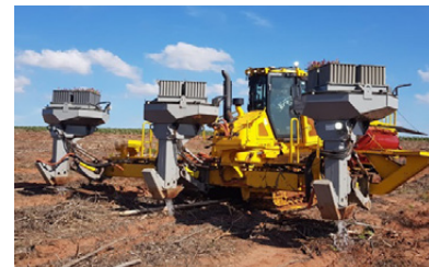
Crawler planter equipped with Bracke-made attachments on Komatsu-made bulldozer
